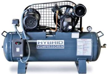
These Hybrid Brand Two Stage Reciprocating Air Compressors are specially designed to cater to the medium pressure application and are made of heavy-duty components to give desired effective output. These compressors have two different sized cylinder bores which increases the efficiency of these compressors.
