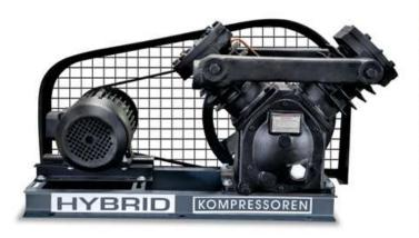
This Vacuum pump has a universal design with the provision to convert it into a single stage compressor. This feature provides a very vital additional facility for large tank leakage test under vacuum or under pressure.
